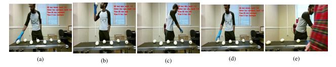
Figure 2: (a–d) These frames show a human picking an onion, inspecting it, placing it after making a decision, and choosing the next onion in sequence. The red text appearing on the images is the state predicted by SA-Net. (e) An example occluded frame where SA-Net is unable to make a prediction. At this point the expert could be placing the onion back on the conveyor or in the bin.
